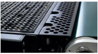
Chip removal system positioned between the machine and the unloading belt, guaranteeing optimal sheet cleanliness.
