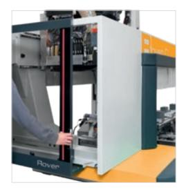
The large hatch, which can be opened, facilitates access for tooling operations and for cleaning the front of the machine.
