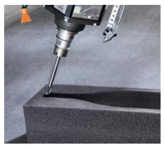
The 5-axis unit with direct drive motor offers maximum flexibility in inclined and interpolated machining operations, with no need to fear excessive stress.
