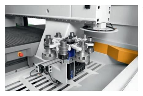
8-position revolver integrated into the machine beam.
