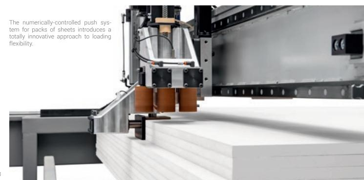
The patented loading system, using collets, allows the loading of books of panels (or highly porous panels) that it would otherwise be impossible to move with the suction cups.
