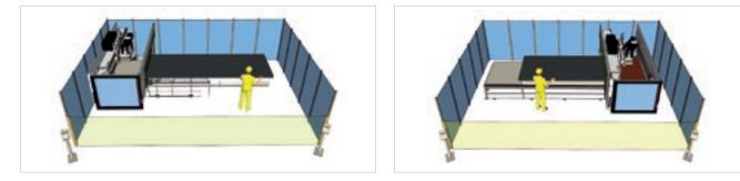
The machine can be configured with tandem loading in order to alternately process sheets. This allows for loading or unloading to be carried out during machining operations.
