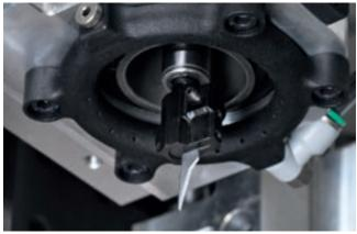
Blower device for cutting units reduces blade overheating and hence the risk of damage to certain types of material, at the same time keeping the cutting area clean and free of dust and other machining waste.
