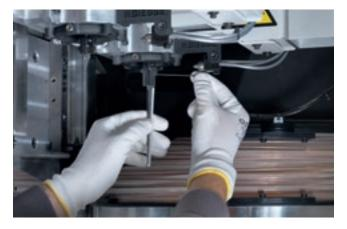
**Extremely quick and simple blade changes** The operator can make a blade change in just a few steps, limiting the machine downtime.
